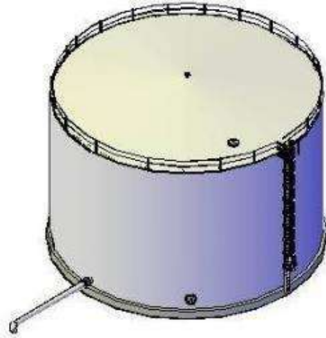
Gambar 2. 1 Fixed Roof Tanks .
